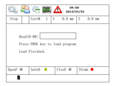
Iuput a mold number 21(0-99), then press key to load the program. The program runs in AUTO mode.
