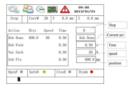
Press key step by step, picker will do the action list one by one. To teach a new action, using manual key to do this action, then press key to confirm the change.
